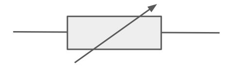
A resistor with variable resistance.
