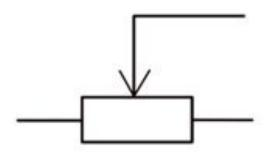
Divide the source voltage into smaller parts to vary the voltage, using resistors.
