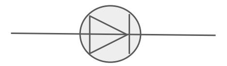
A component which only allows current to flow in one direction (as the resistance in the other direction is too high).
