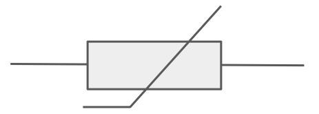
A resistor in which resistance decreases as temperature increases.
