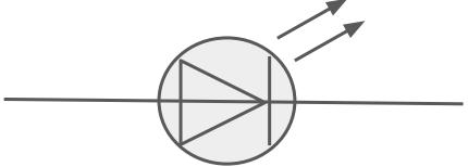
A diode which allow current to flow in only one direction by having high resistance to flow in the opposite direction and emits light in doing so.
