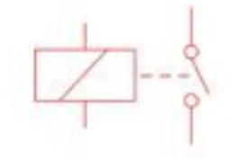
Switches on a circuit with a high current, using a circuit with a small current.
