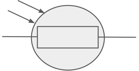
A resistor in which resistance decreases as light intensity increases.
